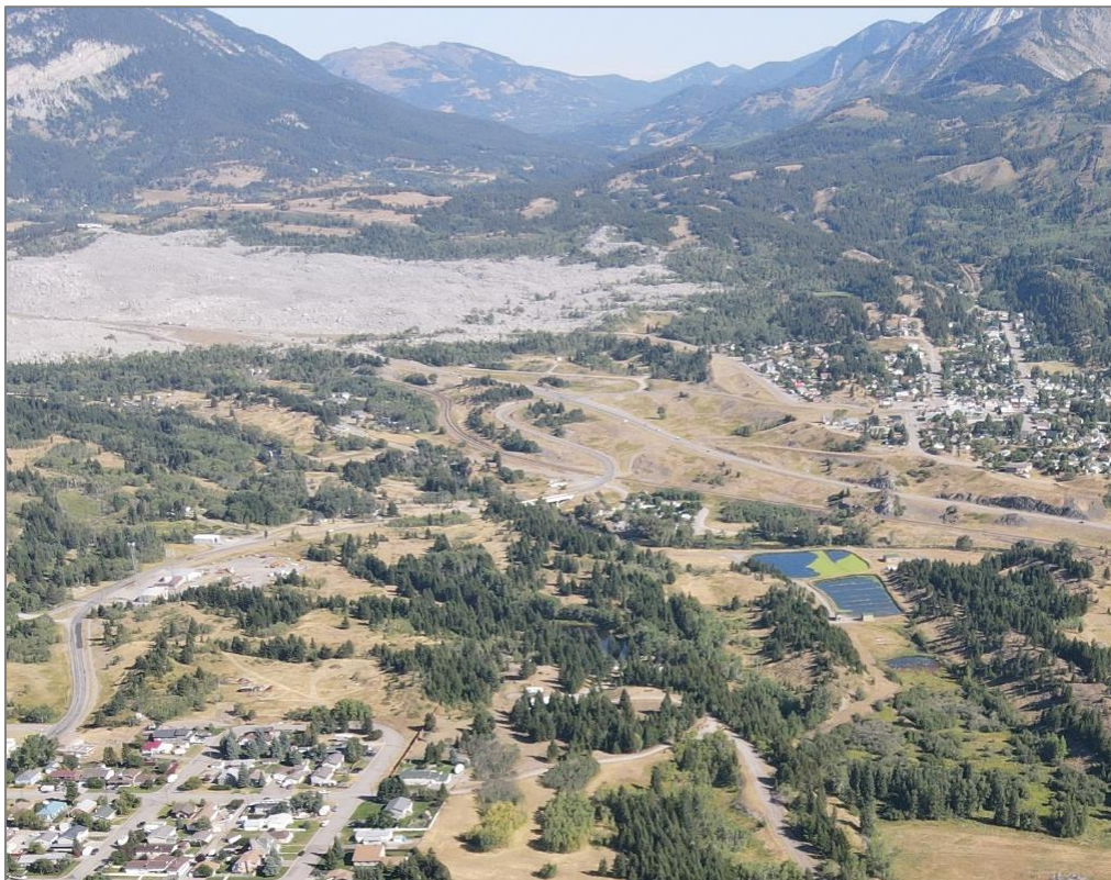
FIGURE 42 - SEWAGE LAGOONS BETWEEN BELLEVUE AND HILLCREST
